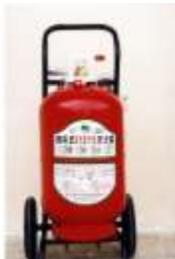
**Halon** extinguishers contain a gas that interrupts the chemical reaction that takes place when fuels burn. These types of extinguishers are often used to protect valuable electrical equipment since they leave no residue to clean up. Halon extinguishers have a limited range, usually 4 to 6 feet. The initial application of Halon should be made at the base of the fire, even after the flames have been extinguished.
